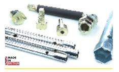
Sink and Tap Back Nut Kit includes 8-13mm monobloc (3240U) and 27x32mm box spanners (319U) for most kitchen and bathroom taps. Also included is the Shorty Handle Basin Wrench (4357G) and of course the Grip+ fittings which connect the head of the Basin Wrench to the box spanners. The kit also contains a 3 prong tool for holding a sink rose/ strainer whilst fitting the waste nut with a 50mm box spanner.
