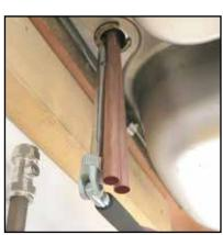
4562P fit box spanners 8-13mm. When used with 345V or 4537G handles gives improved access, extension and leverage.
