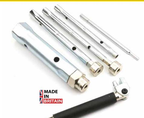
**The Monument Grip+ Tap Back Nut Tools** range from 8mm through 19mm and then additional sizes of 22mm 24mm 27mm and 32mm. The tools are designed to fit existing 345V Professional Adjustable Basin Wrenches as well as the 4537G Shorty Handle Basin Wrench. The unique design of the fitting of the tool simply sanp-fits onto the cast head of the baisin wrench. The other end of the tools engages with the end of the box spanner.
