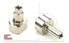
The Monument Grip+ Radiator Bleed Keys come in two different sizes - as vent pins tend to have a habit of not being a consistent size. The 12mm A/F hexagon with 5.3mm Square socket for Radiator Vent Pins (4503L) is found in the Radiator Kit (GRIP4600).
